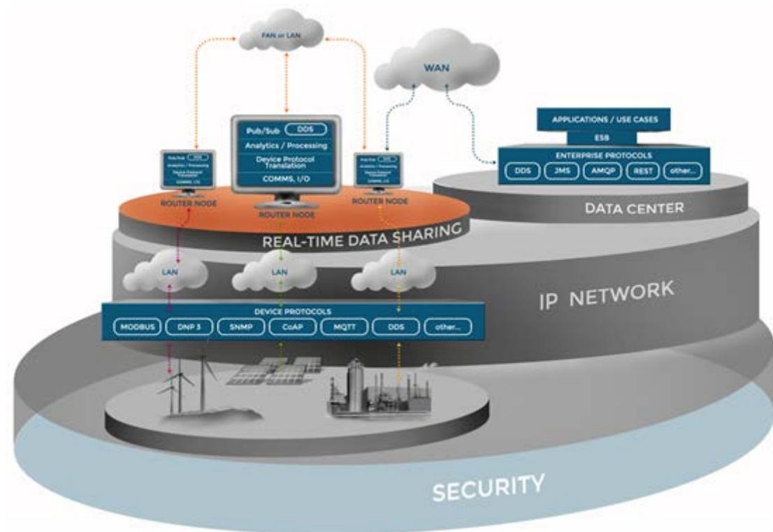
Figure 2 – Layered IIoT System Architecture
