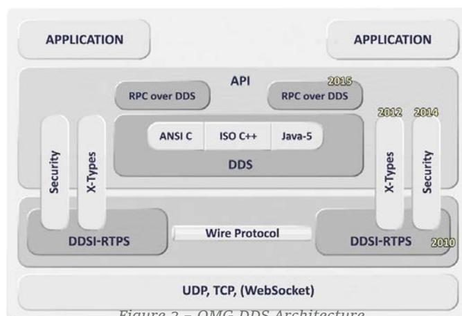
Figure 3 – OMG DDS Architecture
