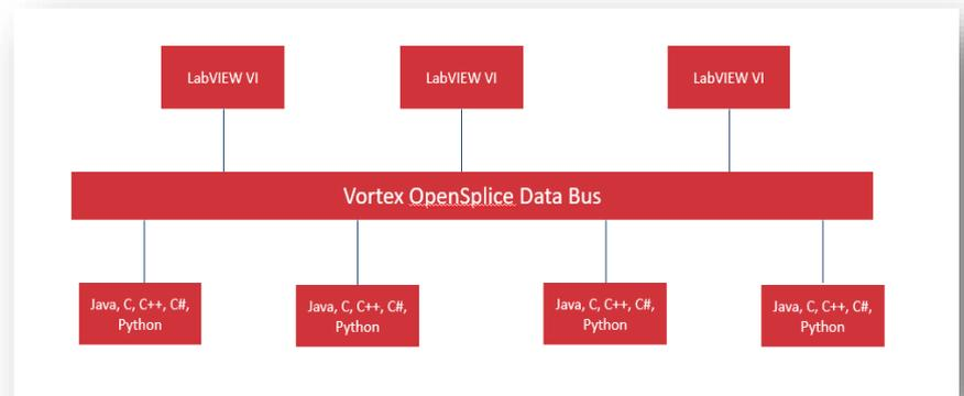
LabVIEW applications can communicate via a publish / subscribe model. Automatic discovery matches publishers and subscribers, routing data accordingly. This significantly reduces the amount of custom code required to support system communications.
